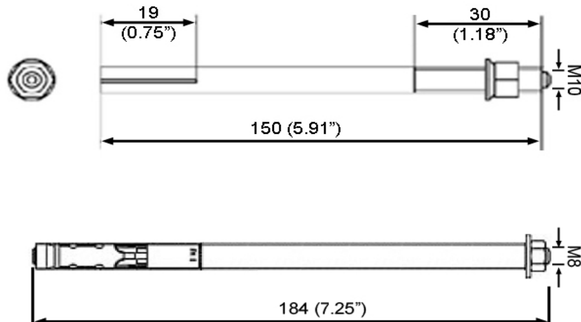
Illustration 2-3: Typical Floor Anchors
